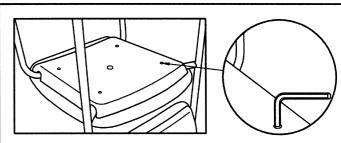
PREVENTIVE MAINTENANCE AND WARNING! • From time to time, check to make sure screws are securely tightened. Delta Holes on PP shell are for convenient checking.
